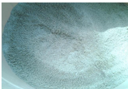
Figure 3b: Picture of fine sand (0.125 mm in diameter) used in slow sand filtration system design (31cm depth).
