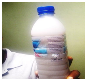
Figure 5a: Picture of untreated salon waste water.
