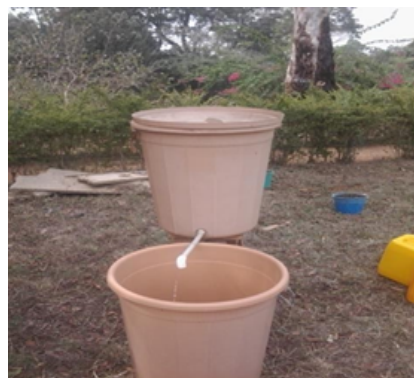
Figure 4a: Picture of the overall set-up of the slow-sand filtration system used for the treatment of salon waste water in Cape Coast.
