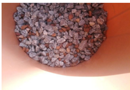
Figure 2b: Picture of gravels (Average 3 cm in diameter) used in slow sand filtration system design (11 cm depth).
