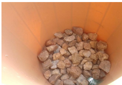
Figure 2a: Picture of stones (Average 6 cm in diameter) used in slow sand filtration system design (8 cm depth).
