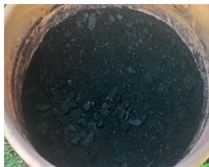
Figure 4b: Picture of Activated Charcoal layer used for the treatment of salon waste water in Cape Coast.
