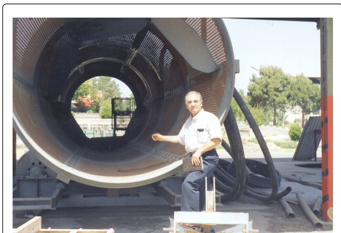
Figure 7: Drum sieves, used to screen garbage through mesh into different size classes for further screening on vibrating conveyors.
