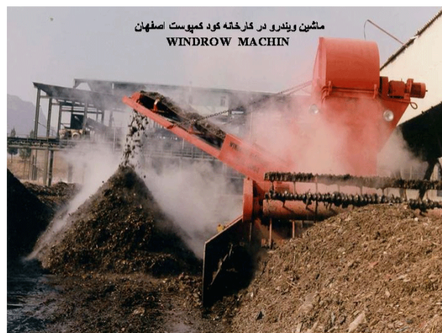
Figure 10: Mixing and turning of organic waste by a compost turner, which turns each windrow every four days.
