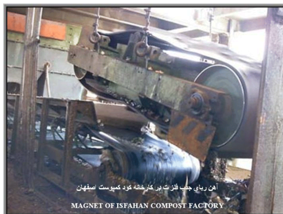
Figure 5: Magnets used to separate metals from the remainder of the waste stream.
