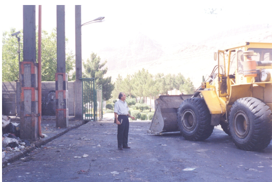
Figure 3: A large front-end loader pushes the garbage to the conveyors, immediately and cleaning the drop-off site.
