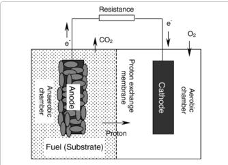
**Figure 1:** Classical dual-chamber MFC with a bioanode and an oxygen cathode (figure reprinted from [3] with permission from Elsevier).
