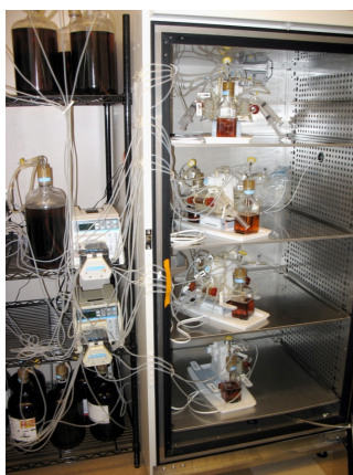
Figure 6: Typical laboratory set up of the hollow fiber two compartment model. The large volumes of diluent and the waste reservoirs are kept outside the incubator. Micro-processor controlled peristaltic pumps add and remove the diluent from the central reservoir inside the incubator. Sampling is performed via the side ports on the hollow fiber cartridge.
