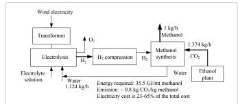
Figure 5: Schematic of methanol production using renewable hydrogen and CO, [13,22,63].
