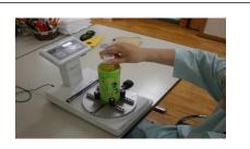
**Figure 1:** The equipment used and measurement position. Digital Torque Meter 2TME450CN (N·cm), c, Co., Ltd.
