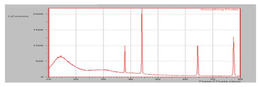
Figure 10: Diffractogram of citric acid.
