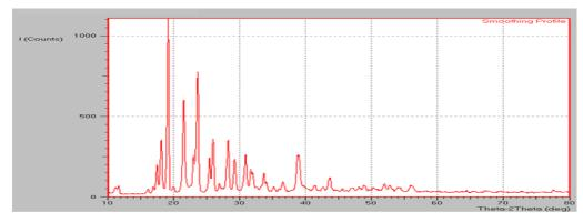
Figure 9: Diffractogram of pure ritonavir.
