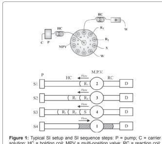
solution; HC = holding coil; MPV = multi-position valve; RC = reaction coil; D = detector; W = waste; R, & R, = reagents; S = sample; S1-S4 = SI steps.
