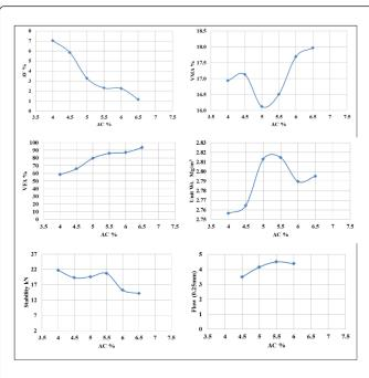
**Figure 4:** Marshall test graphs for 50% steel slag + 50% gabbro asphalt concrete mixture.
