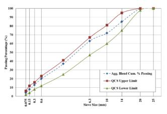
Figure 1: Design Gradation and QCS-2010 Limits.
