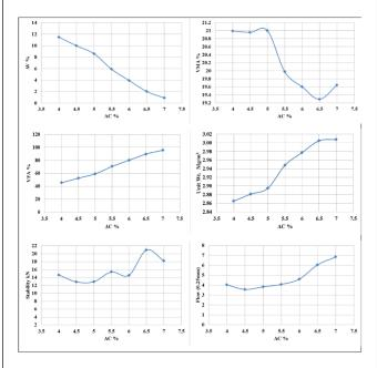
**Figure 3:** Marshall Test graphs for 100% steel slag asphalt concrete mixture.
