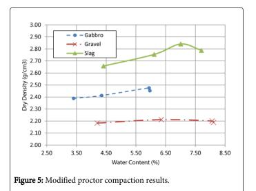
Figure 5 indicates that the optimum moisture contents for steel slag, gravel and gabbro aggregates are 7.0%, 6.4% and 5.9%, respectively. The largest dry density was achieved in the steel slag aggregates.
