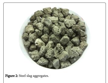
The steel slag, gravel and gabbro aggregates failed the liquid limit and plastic limit tests (i.e. the aggregates are non-plastic). In addition, the bulk, saturated surface-dry (SSD) and apparent (APP) specific gravity tests were performed on the steel slag, gravel and gabbro aggregates. Table 2 indicates that all specific gravity values for steel slag (fine and coarse) are greater than those of gabbro and gravel.
