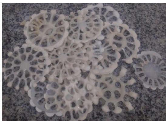
Figure 2: PMMA-based dental resins scraps in form of rosettes, discharged by the quality production process control, were used as raw material by depolymerization at 350 °C, 400 °C, and 450 °C, 1.0 atm. in laboratory scale.
