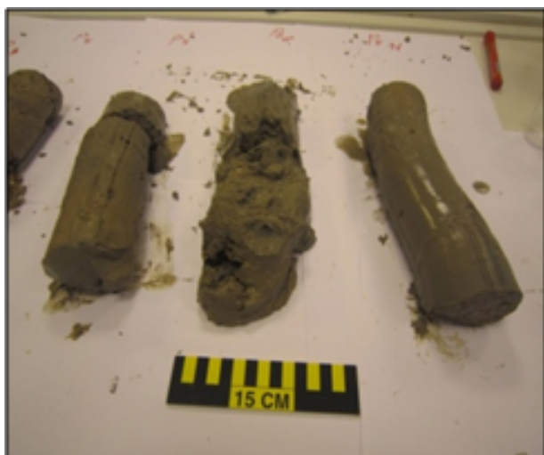
Figure 8: Cores samples obtained from hand-held corer.
