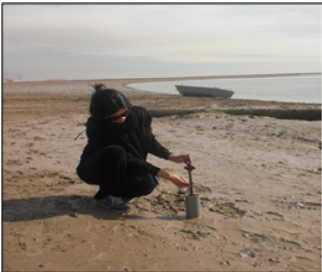
Figure 7: Sampling by hand-held corer on the tidal flat.
