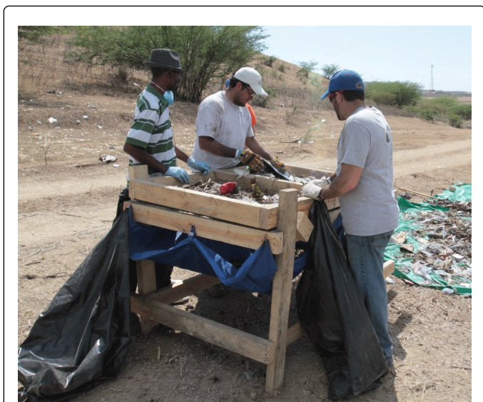
Figure 2: The sieve-shaker table designed and used for rapid waste composition studies.
