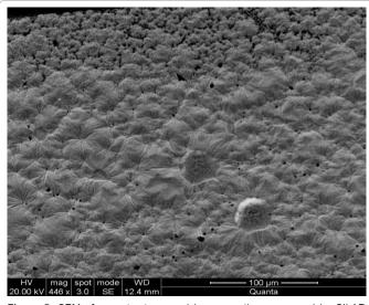
Figure 5: SEM of nanostructure seed layer growth on prepared by SILAR method using ICON Anakytical (FET QUANTA 200) Scanning Electron Microscope.
