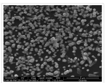
Figure 6: ZnO nanostructure of CBD growth SEM image.
