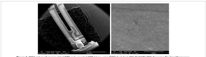
Figure 1: SEM picture of encapsulated QTF and uncoated QTF taken using ICON Analytical (FEI QUANTA 200) Scanning Electron Microscope.
