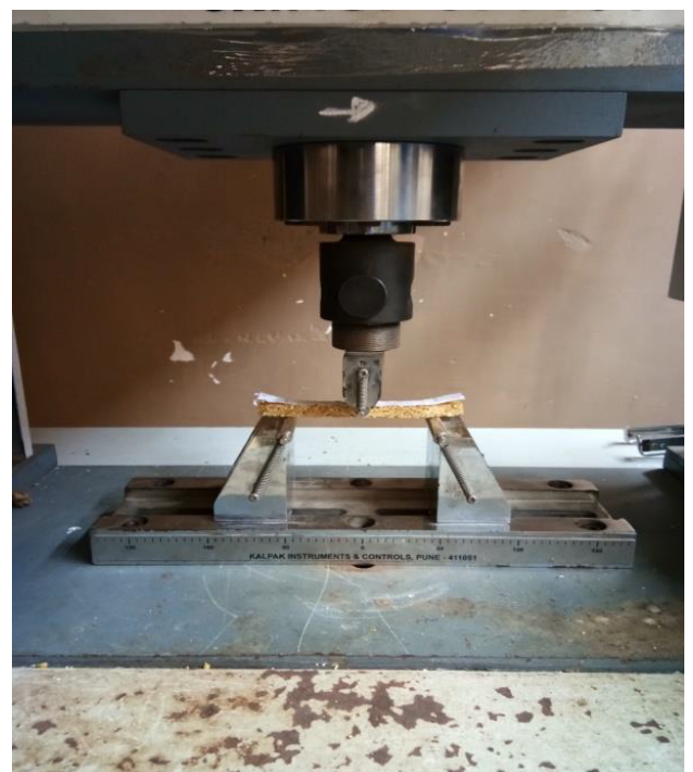
Figure 19: Setup and bending test of specimen A.
