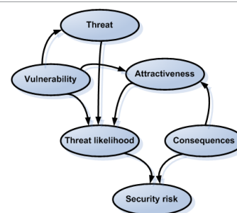
Figure 1: Schematic relation among different parts of a security risk analysis. The arcs imply the causal relationships.
