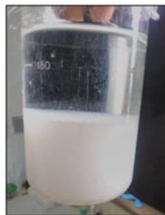
Figure 7: Residu solution after addition of 1M HCl.
