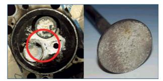
Figure 1: Deposits on the generator valves.
