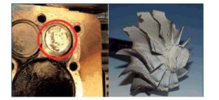
Figure 2: Incrustation on valves and turbines.
