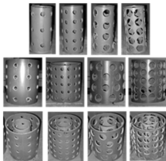
Figure 2: Cylinder model –D1 (top), D2 (middle) and D3 (bottom), left to right – porosity, P = 0.0625, 0.14, 0.28 and 0.48 , respectively.
