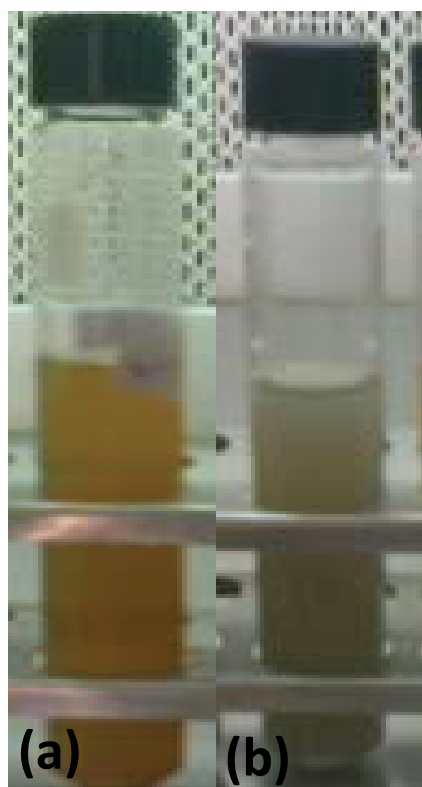
Figure 1: Change in color of fungal filtrate (a) before \text{AgNO}_3 (b) after addition of \text{AgNO}_3 .
