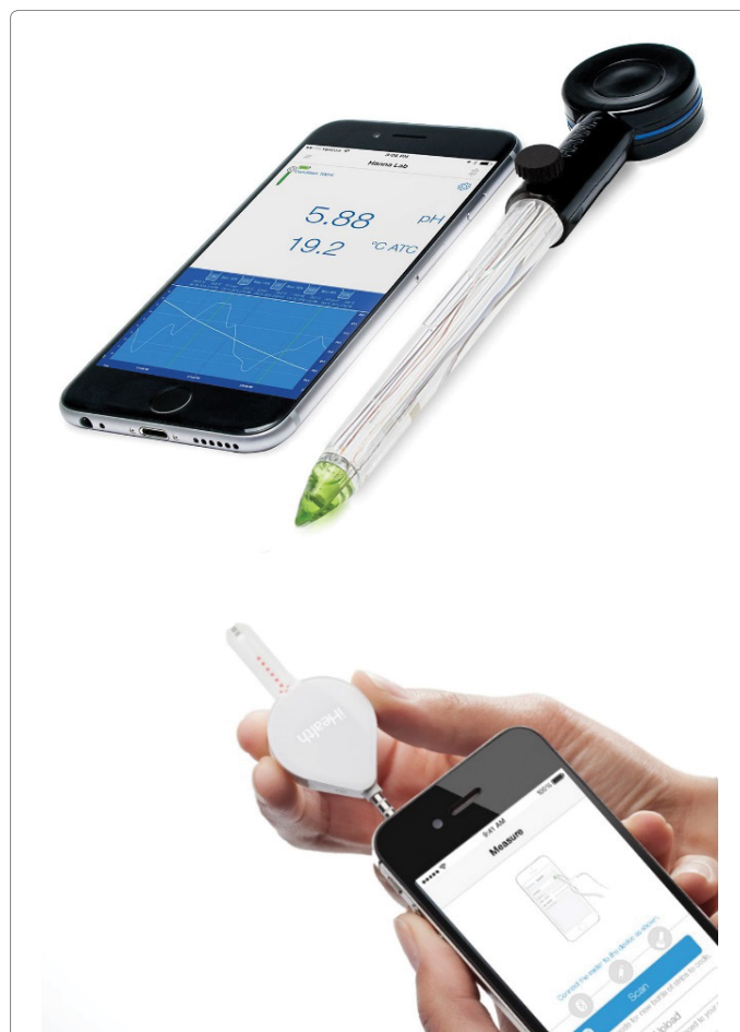
Figure 1: The examples of commercially available mobile-phone-based portable analytical devices: A - The pH probe with Bluetooth technology ( http://hannainst.com/halo ), B - The electrochemical portable glucose meter employing blood glucose test stripe, which plugs directly into the smartphone's headphone jack, and displays results directly on the phone screen [11].
