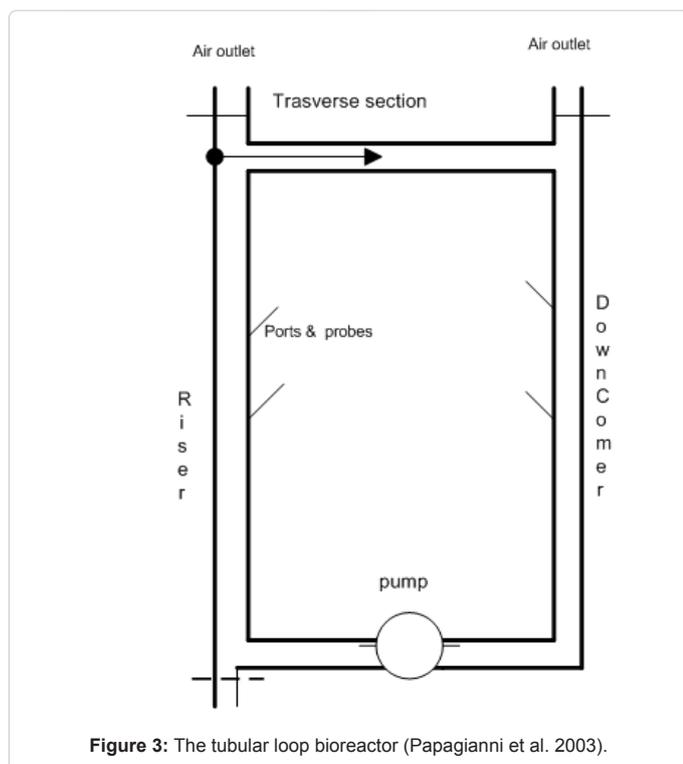
Figure 3: The tubular loop bioreactor (Papagianni et al. 2003).
