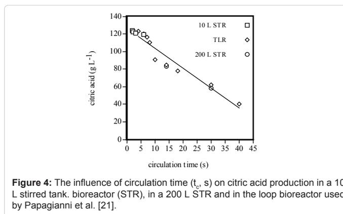
Figure 4: The influence of circulation time ( $t_c$ , s) on citric acid production in a 10 L stirred tank bioreactor (STR), in a 200 L STR and in the loop bioreactor used by Papagianni et al. [21].
