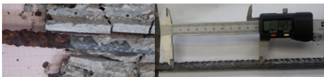
Figure 5: View of the protruding area of a specimen (left), view of the bare area of a specimen (right).
