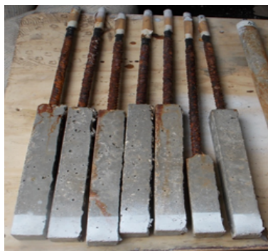
Figure 3: View of corroded rebars.
