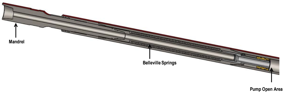
Figure 5: Shock tool or oscillation section of an axial oscillation tool (AOT).
