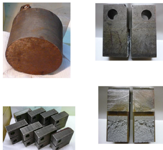
Figure 2: Steps of 1T-CT type specimens from 140 mm in diameter EPR RPV trepanmanufacturing (left side) and testing.
