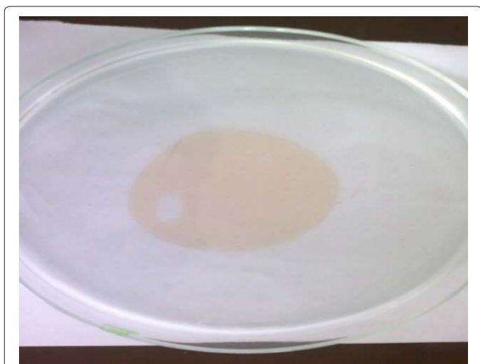
Figure 8: Oil displacement by biosurfactant. The area displaced can be seen as whitish halo within the oil spread.
