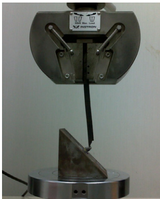
Figure 2: The metal base used to hold the specimen for testing.
