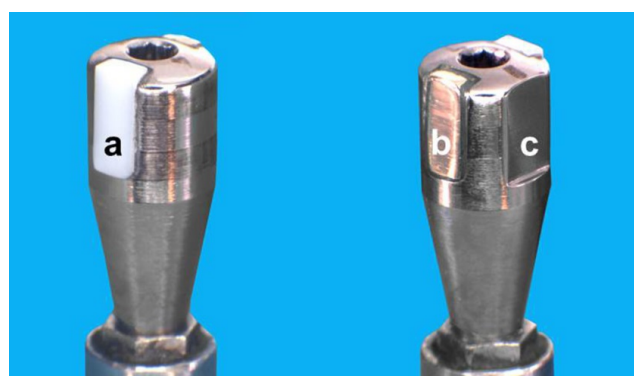
Figure 2: Modified healing abutments with a zirconia sample (a), a gold sample (b) and a polished titanium surface (c).
