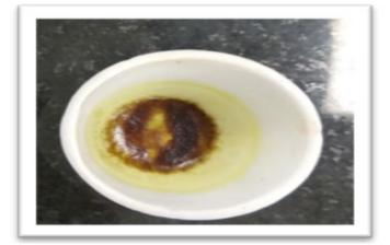
Figure 4: Dried sample in crucible.
