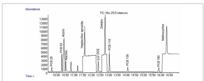
Figure 2: Extract of Reagent Water Spiked with, 3.966 µg/L Aldrin, 2.368 µg/L of Alachlor, 10.416 µg/L of Heptachlorepoxide, 12.800 µg/L of Dieldrin, 20.956 µg/L Methoxychlor, 1.413 µg/L p,p' - DDE, 0.498 µg/L PCB 28, 0.436 µg/L PCB 52, 1.830 µg/L PCB 118, 0.619 µg/L PCB 138 and 0.115 µg/L PCB 180.
