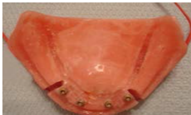
Figure 1: Model 2 with ERA mini implant having the strain gauge wires attached to the model.
