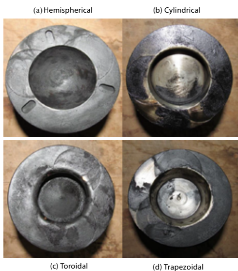
Figure 3: Combustion chamber shapes.
