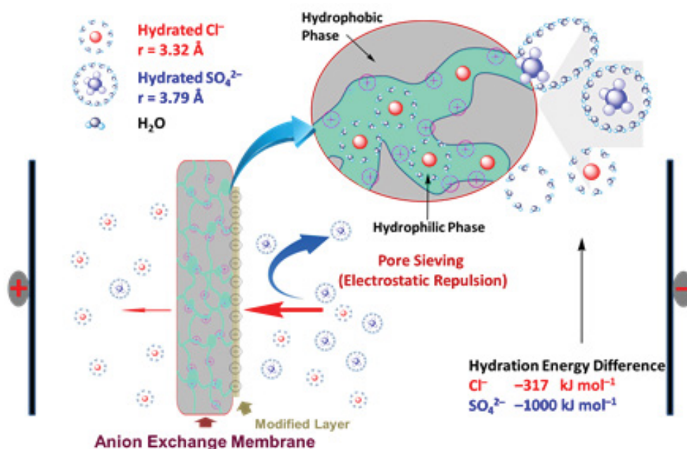
Figure 2: The proposed possible mechanisms of MASMs in ED process (Cl - /SO 4 2- solution system as an example).
