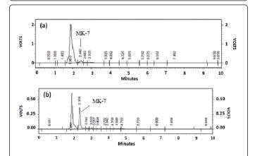
Figure 3: The chromatograms of extracted MK-7 from soybean nutraceutical by propan-2-ol and n-hexane (1:2 v/v) solvents without (a) and with internal standard (b) of concentration 2.5  $\mu g$  mL<sup>-1</sup>.
