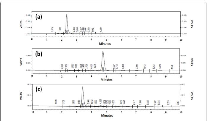
**Figure 1:** The chromatograms of MK-7 (10  $\mu$ gmL<sup>-1</sup>) eluted under chromatographic conditions I (a), chromatographic conditions II (b) and chromatographic conditions III (c)
