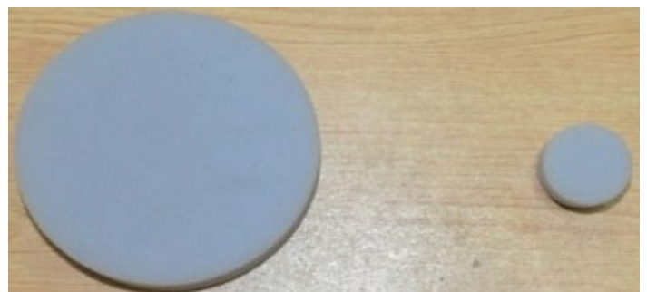
Figure 5: Testing samples of melamine foam (100 mm & 30 mm diameters).
