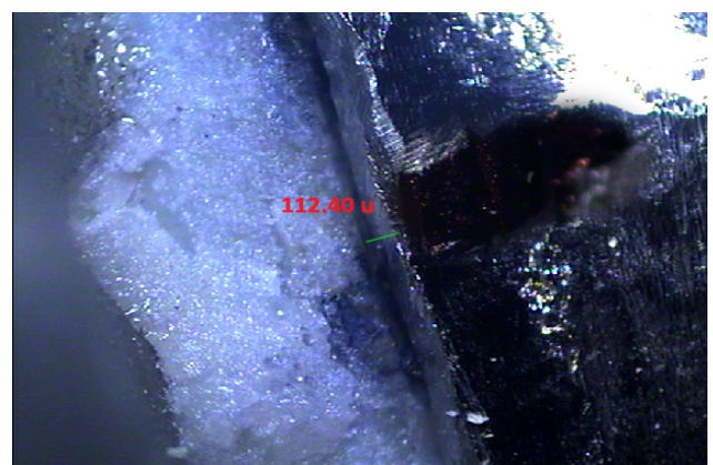
Figure 12: Photograph showing marginal discrepancy of group IIa sample as seen under the stereomicroscope.
