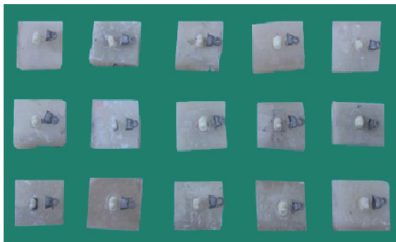
Figure 16: Photograph showing dislodged metal copings of group I.
