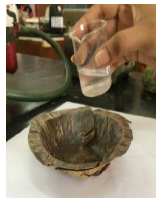
Figure 19: Checking the water holding capacity after the coating.
