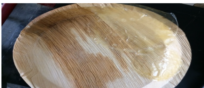
Figure 5: Chitosan based film with (Turmeric essential oil) at the concentration of 0.4 g Chitosan.
