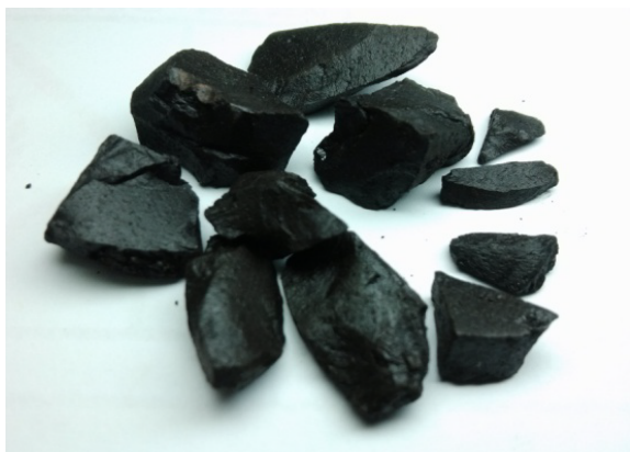
Figure 2: Trinidad Lake Asphalt (TLA).
