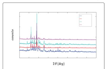
**Figure 1:** The XRD spectra from SAMPLE 1, 2, 3 and 4 showed similar features corresponding to a mostly composition of Anorthite Sodian composition. For claritythe spectra have been shifted 2000 units from SAMPLE 2. The presence of magnetite in SAMPLE 1 is denoted as peaks around 50 (deg).
