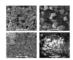
**Figure 2:** Representative SEM micrographs (Magnification 150X) obtained from (a)-(d) the SAMPLES 1, 2, 3 and 4 respectively. The images show mostly fragmented materials in all the samples analyzed.
