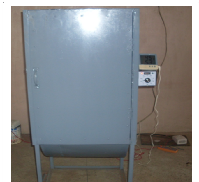
Figure 3: Pictorial view of the dryer showing the temperature regulator.
