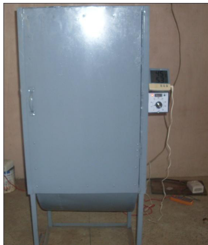
Figure 3: Pictorial side view of the dryer showing the temperature regulator.
