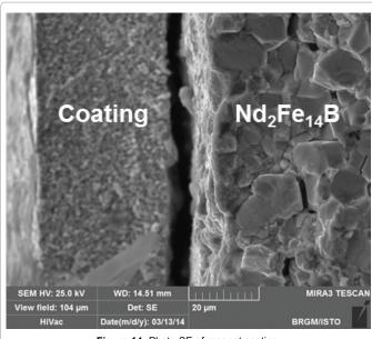
Figure 14: Photo SE of magnet coating.
