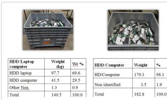
Figure 7: Hard disks drive representative sample.
