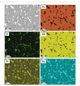
**Figure 15:** Textural and chemical characterization of a HDD permanent magnet after demagnetization.
