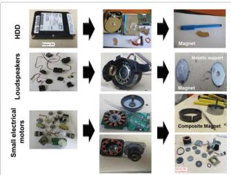
Figure 8: Recovery of magnets from different electronic components of WEEE by manual dismantling.
