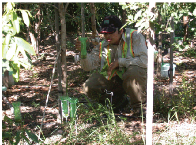
Figure 5: Standard rain gauge used in measuring throughfall.
