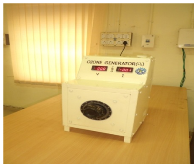
Figure 6: PEM ozone generator.
