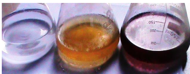
Figure 3: Showed the synthesis of Nanoparticles. (a) - 1 mM Silver Nitrate solution, (b) - Seaweed extract, (c) - Biosynthesized Silver Nanoparticles.
