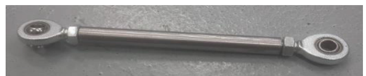
Figure 5: Rod replacing dampers.
