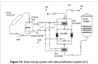
dehumidification (adsorption) process, the air inside the dryer passes through the heat exchanger by use of the blower. However, since no hot water is circulated in the heat exchanger, the air reaches the adsorbent. The air is dehumidified with the adsorbent and is supplied the drying load as the dry air. The relative humidity and temperature of the drying chamber were 40% and 35°C respectively.
