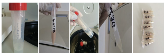
Figure 2: Purification through the column (pD-10 desalting columns contain Sephadex G-25)
