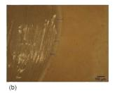
Figure 2: Marginal discrepancies of the zirconia cores that were made by (a) a CAD/CAM system and (b) a copy milling system. These light microscopic views show that the copy milling system produced more accurate zirconia cores than the CAD/CAM system did.
