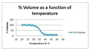
**Figure 2:** The volume change of a poly(N-isopropylacrylamide) microgel in water as a function of temperature.
