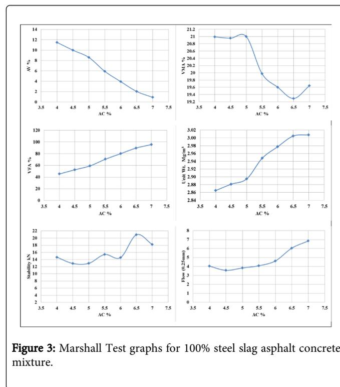
**Figure 3:** Marshall Test graphs for 100% steel slag asphalt concrete mixture.
