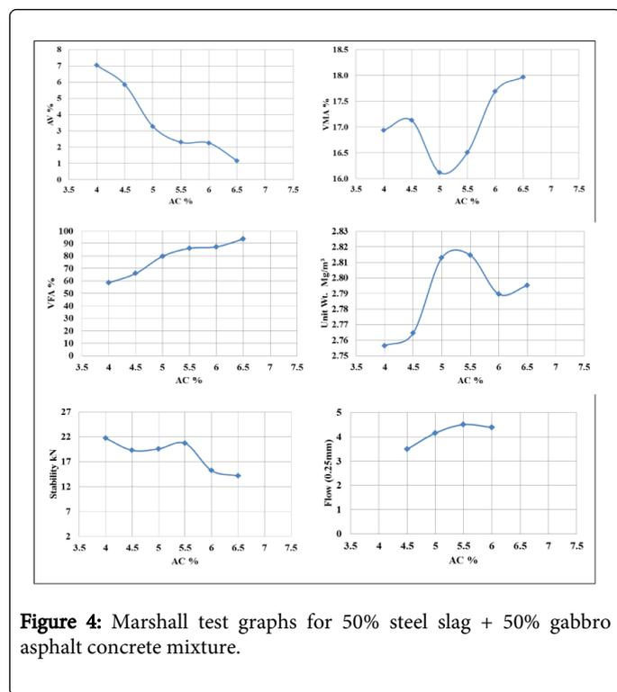
Figure 4: Marshall test graphs for 50% steel slag + 50% gabbro asphalt concrete mixture.
