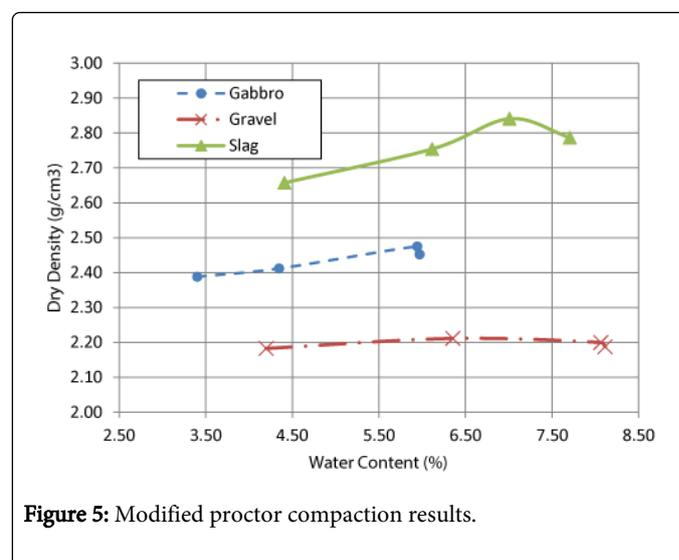
Figure 5: Modified proctor compaction results.
