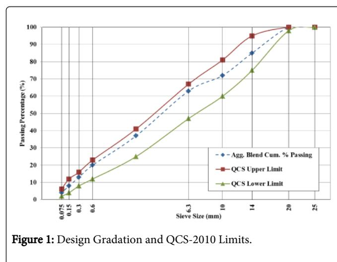
Figure 1: Design Gradation and QCS-2010 Limits.
