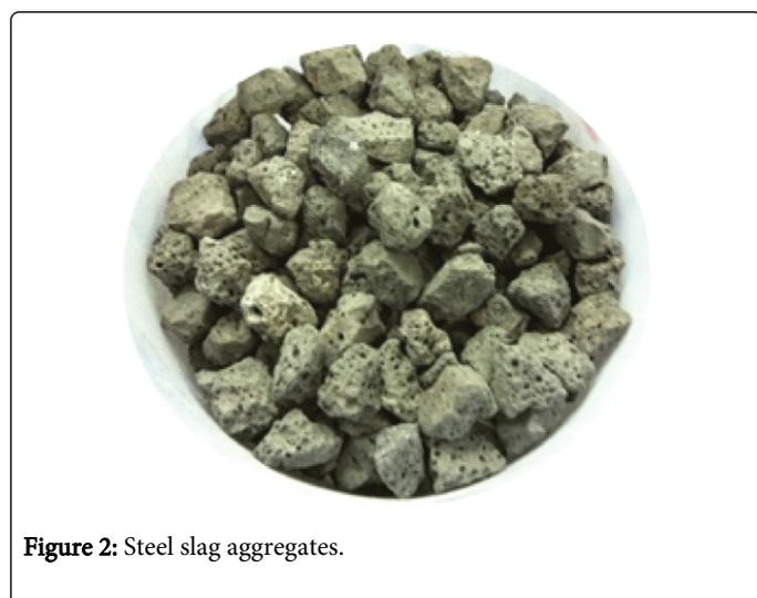
**Figure 2:** Steel slag aggregates.
